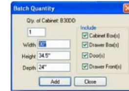
Simply select a cabinet from the included library right at the machine control, adjust the size and cut it. Extensive libraries of cabinets and closets are included and these can be modified or new libraries created using a programming service from Thermwood. All the cabinet shop has to do is run.
